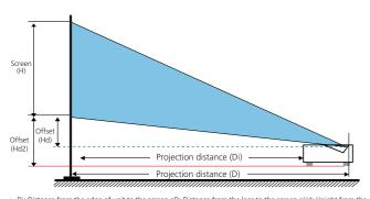
Di: Distance from the edge of unit to the screen •D: Distance from the lens to the screen •Hd: Height from the center of lens to the bottom of screen \*Hd2: Height from the projector mounting surface to the bottom of screen
